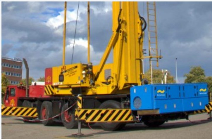
Electriq Hydrogen Powder powering a mobile crane, Sep 2022, Rotterdam
